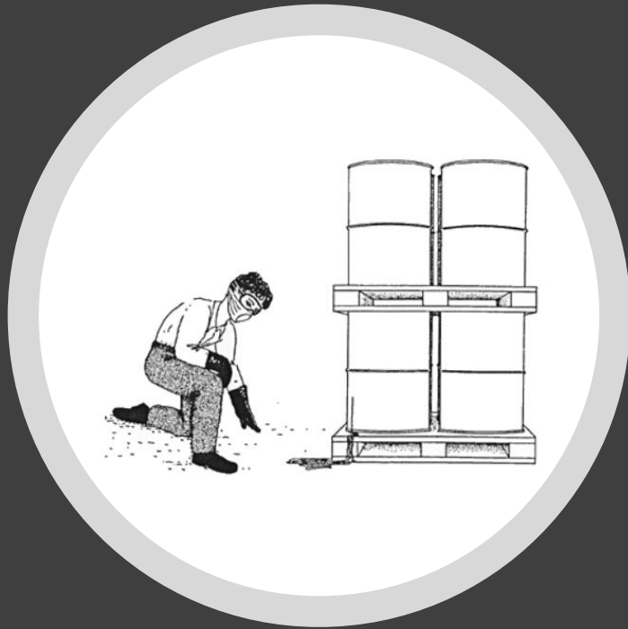
Leak from container
